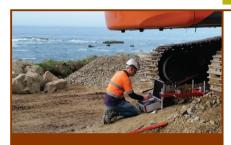
Static plate load testing for performance based design of pavements and stone columns
